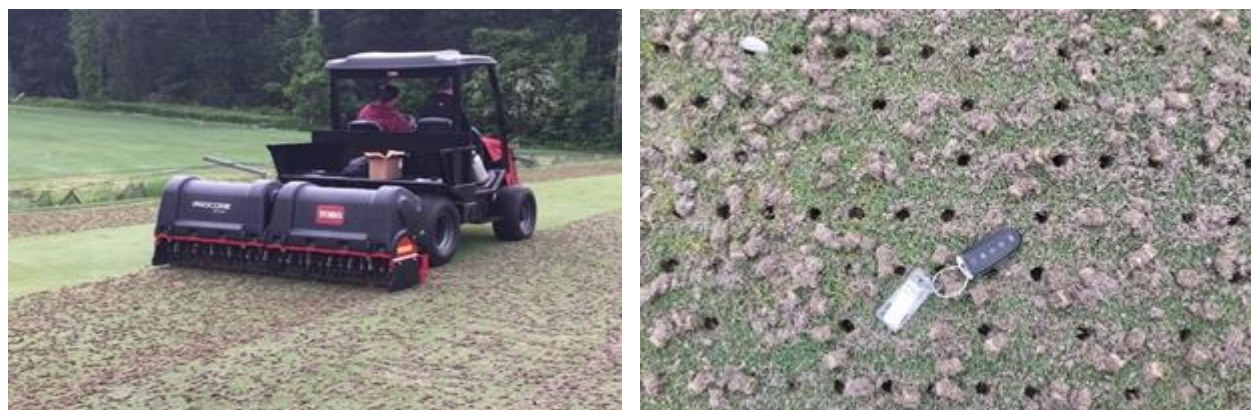
Figure 6-8. Hollow-tine cultivation on a tee at West Point Golf Course in West Point, NY.
