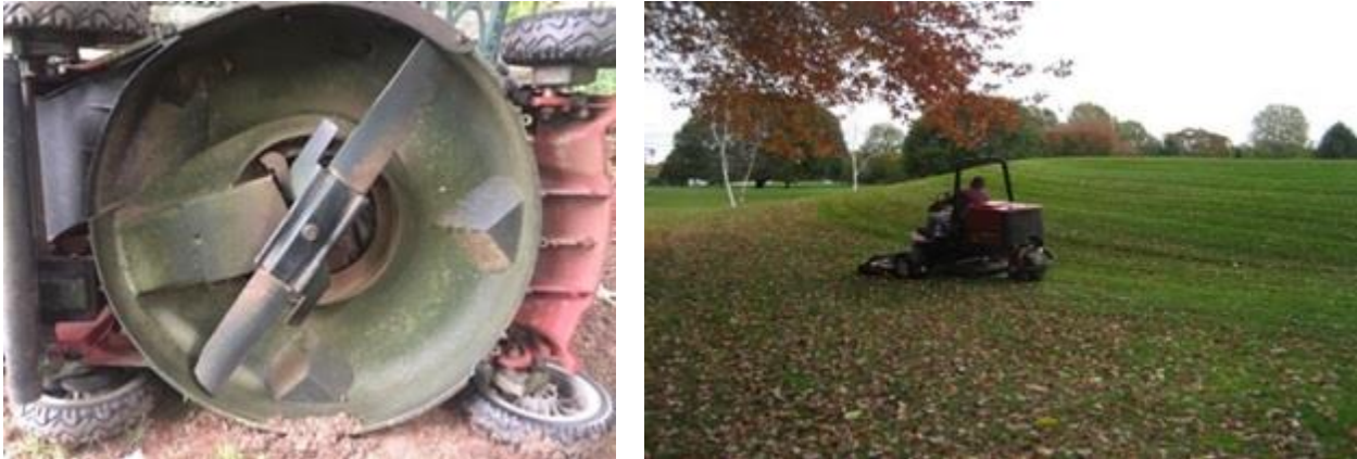
Figure 6-4. Rotary mowers are used for rough and surrounds (bunker, green, and tee). Sharp rotary blades are necessary for a quality cut and plant health.
