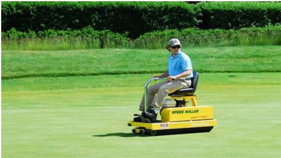
Figure 6-7. Rolling putting green surfaces can allow managers to reduce mowing frequency or raise mowing heights while maintaining putting green speeds.
