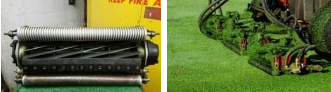
Figure 6-3. Reel mowers are used on greens, collars, tees, approaches, and fairways. Proper reel to bed knife adjustment is necessary to maintain plant health.
